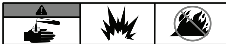
Battery acid is corrosive, explosive and flammable
