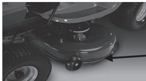
Stamped Deck Shell below, NOT reinforced
