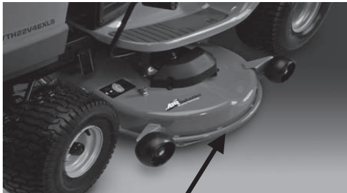
Armor Protected Stamped Deck Shell Example Below
