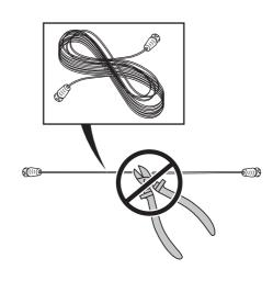
It is possible to let the low voltage cable cross the working area. The low voltage cable must be stapled down or buried, and the cutting height should be such that the blades on the blade disc can never come in contact with the low voltage cable.
