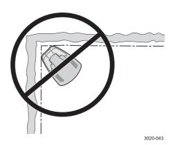
The charging station must be positioned on relatively level ground. The front end of the charging station must be a maximum of 1.2" (3 cm) higher than the back end. The front end of the charging station must never be lower than the back end.
