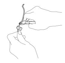
4. Press the connector onto the metal pins, marked with an A, on the charging station.
