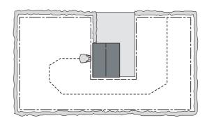
When the battery is fully charged, the robotic lawnmower leaves the charging station in a randomly selected direction within the 90°-270° exit sector.
