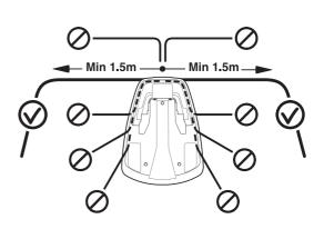
The charging station must be positioned with a great deal of free space in front of it (at least 10 ft [3 m]). It should also be centrally placed in the working area to make it easier for the robotic lawnmower to reach all areas in the working area.
