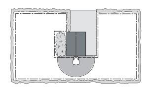
Do not put the charging station in confined spaces in the working area. There must be a straight boundary wire, at least 5 ft (1.5 m) long, to the right and left of the charging station. The wire must be laid straight out from the rear end of the charging station. Any other locations can mean that the robotic lawnmower enters the charging station sideways and will have difficulty docking.
