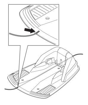
2. Fit the connector to the guide wire in the same way as for the boundary wire described in 3.5 Connecting the boundary wire. Connect it to the contact pin on the charging station that is labelled 'Guide'.
