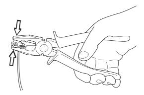
3. Cut off any excess boundary wire 0.4"-0.8" (1 or 2 cm) above each connector.
