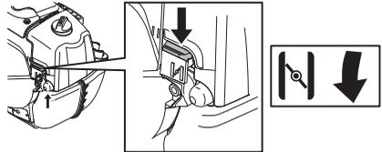
Hold the body of the machine on the ground using your left hand (CAUTION! Not with your foot!). Grip the starter handle, slowly pull out the cord with your right hand until you feel some resistance (the starter pawls grip), now quickly and powerfully pull the cord.
