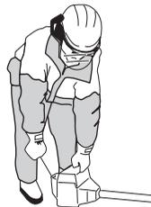
**CAUTION!** Do not put any part of your body in marked area. Contact can result in burns to the skin, or electrical shock if the spark plug cap has been damaged. Always
