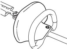
Check that the hand guard is fitted correctly.
