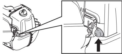
**Choke:** Set the choke control in the choke position.
