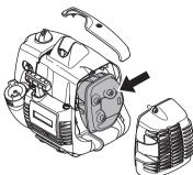
Some mufflers are equipped with a special spark arrestor screen. If your machine has this type of muffler, you should clean the screen at least once a week. This is best done with a wire brush.
