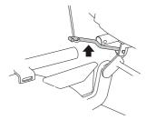
3 Push the cutting deck in and make sure the guide bolts fit into the grooves on the deck frame, one on each side.
