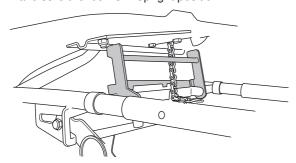
10 Remove the pin in the equipment frame.
