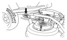
4 Fit the cutting deck's pipe together with the deck frame's pipe.
