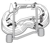
Lock the blade with a wooden block. Loosen the blade bolt and remove the blade bolt, the washer and the blade.
