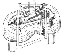
10 Tension the belt with the belt adjuster.
