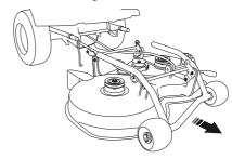
12 Lift off the deck and lean it against the machine or a wall.
