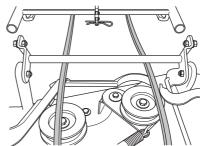
Make sure the lifting lever comes above the cutting deck grip.
