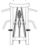
If necessary, the wires can be adjusted by tightening the adjuster nuts on each side of the steering collar. Do not over tighten the cables; they should only be drawn in towards the steering collar.
