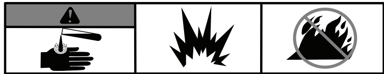
Battery acid is corrosive, explosive and flammable
