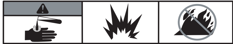
Battery acid is corrosive, explosive and flammable
