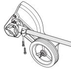
Tighten the two screws.
