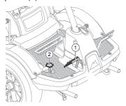
4 Select the required cutting height (1-5) using the cutting height lever.
