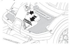
3 M105-85F Pull back the throttle and move the gear shift lever to "N" – neutral position. Turn the ignition key to the "STOP".
