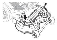
10 Set the cutting deck height control in any of the positions
