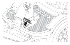
5 Release the clip on the right side of the mower deck and lift the cover off the mower deck.
