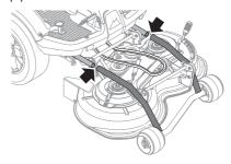
5 Push the cutting deck in and make sure the guide bolts fit into the grooves on the deck frame, one on each side.
