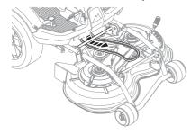
3 Check that the lever for setting the cutting height is in the S position.
