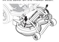
6 Disengage the spring for the drive belt tensioning wheel.
