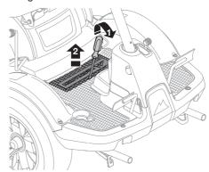
To put back the cover, it must first be bent and inserted at the sides The press down the cover.
