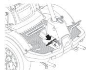
The brake and clutch are engaged by pressing down the pedal entirely. The clutch pedal disengages the engine and stops propulsion. The blade drive is not affected by the clutch pedal.
