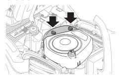
3 Lift out the air filter cartridge from the fan housing.
