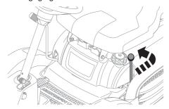
2 Lift up the cutting deck by stepping on the lifting pedal and pressing in the lock button.
