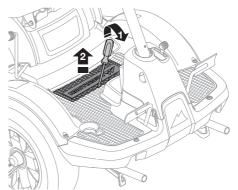
2 Lubricate the drive chain with engine oil or other good quality oil. This is required every 10 hours of running time to maintain full functionality and service life.
