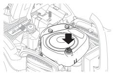
The dipstick should be completely screwed down
