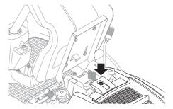
Check that the cooling intake is free from leaves, grass and dirt.
