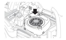
A blocked cooling intake will interfere with the cooling of the engine, which can damage the engine.
