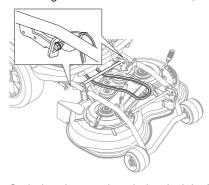
6 Grab the pipes and push the deck in. Push the deck until you feel the pipes touch bottom.
