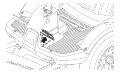
The pedal can also be used to temporarily adjust the cutting height, such as when passing a minor bump in the lawn.
