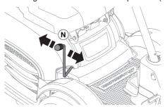
Move the throttle to position 3 (choke position). In this position the engine is fed with a richer mixture, which means the engine is easier to start.
