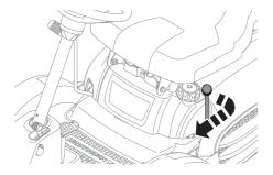
Move the lever back and lock it to stop the blades from rotating.
