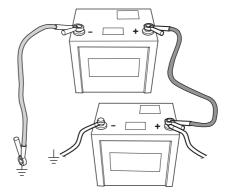
Connect each end of the red cable to the POSITIVE pole (+) on each battery, exercise care not to short circuit any of the ends against the chassis.
