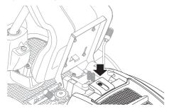
2 Loosen the knobs holding the filter cover in place and remove it.
