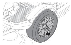
**IMPORTANT INFORMATION** Different tyre pressures on the front tyres will result in the blades cutting the grass at different heights.
