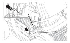
· Push in the control to engage to the drive system.
