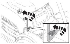
IMPORTANT! Gear changes between forward gears must not be made while the machine is moving.
