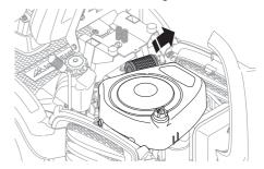
4 Replace the air filter cartridge, if clogged with dirt.
