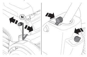
4 When the ride-on mower is at a standstill, engage the parking brake.
