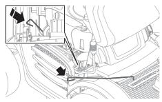
2 Make sure the blades are not rotating by sliding the lever backwards and locking it in the locked position.
