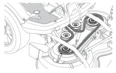
8 Tension the belt with the belt adjuster.
