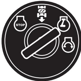
Ⓒ Let the ignition key return to the "ON" position when the engine has started. Push the gas control to the required speed. For cutting: full gas.
