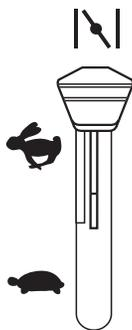
Ⓒ Cold motor: Push the gas control up to end position choke (↖).
