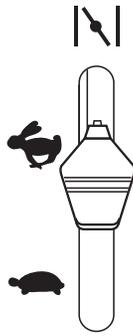
Ⓒ Warm motor: Push the gas control half-way to full gas position "I".
