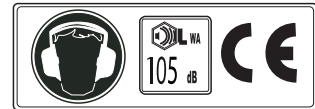
Noise emissions to the surroundings in accordance with the European Union's directive. The machine's emission is stated in the chapter TECHNICAL DATA and on the decals.
