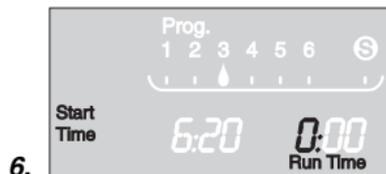
6. Set the hours for the watering time with the **+**-key (example: **0** hours) and confirm with the **OK**-key.
