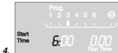
4. Set the hours for starting the watering time with the **+**-key (example: **6** hours) and confirm with the **OK**-key.
