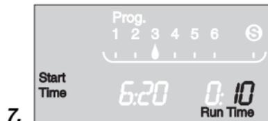
7. Set watering time minutes with the **+**-key (example: **10** minutes) and confirm with the **OK**-key.
