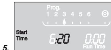
5. Set the minutes for starting the watering time with the **+**-key (example: **20** minutes) and confirm with the **OK**-key.
