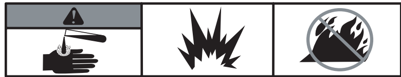
Battery acid is corrosive, explosive and flammable
