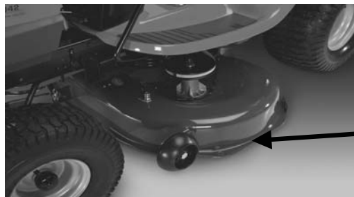
Stamped Deck Shell below, NOT reinforced
