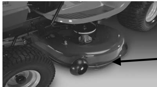
Stamped Deck Shell below, NOT reinforced
