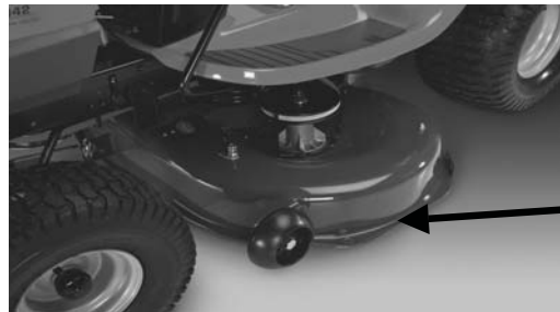
Stamped Deck Shell below, NOT reinforced
