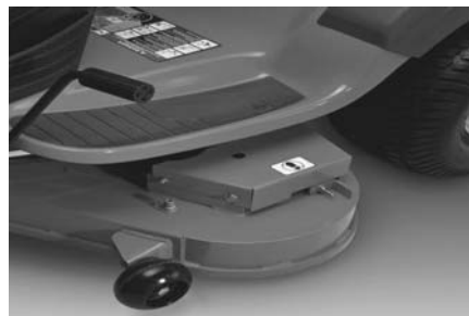
Fabricated Deck Shell Example Below
