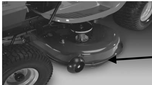
Stamped Deck Shell below, NOT reinforced
