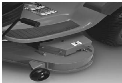
Fabricated Deck Shell Example Below
