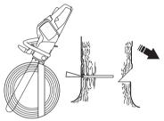
Finish the felling cut parallel with the directional cut line so that the distance between them is at least 1/10 of the trunk diameter. The uncut section of the trunk is called the felling hinge.
