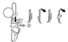
The directional cuts should run 1/4 of the diameter through the trunk and the angle between the top cut and bottom cut should be 45°.
