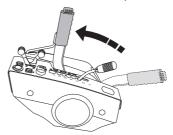
If the cutting unit is left in the lower position, the start lock circuit will prevent engine starts.
