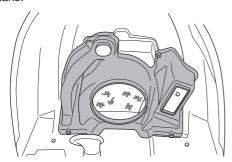
A blocked cooling intake will interfere with the cooling of the engine, which can damage the engine.
