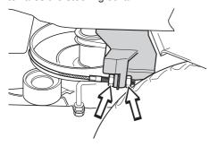
4 Unscrew the belt shields and the side protectors. The protectors are fitted on both sides of the machine.
