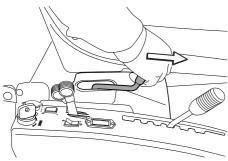
4 Select the required cutting height (1-10) with the cutting height lever.
