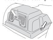
Cooling is impaired if the air intakes are blocked or the transmission housing is dirty, this can result in damage to the transmission.
