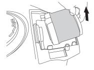
4 Remove the foam rubber prefilter which is placed around the filter cartridge and clean using a mild detergent. Squeeze it dry in a clean cloth.
