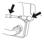
Press the pedal a few times, lubricate again and refit the rubber casing.
