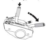
If this does not happen it is probably because the unit has been lifted with the hydraulic lifting lever. Lower the unit to the mowing position with the lever for the hydraulic lift.
