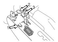
The lights are switched on and off using the power switch (1) on the control panel.
