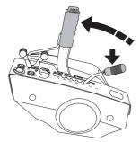
3 Remove the front hood by removing the pin. (There are complete instructions on using the service position inside the front hood).
