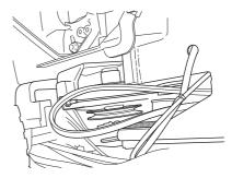
Remove the cooling fan, it is held in place by a nut.
