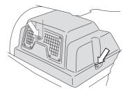
Lubricate the joints and bearings on the left side with oil.
