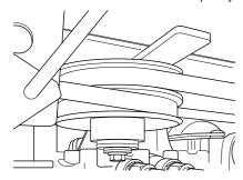
3 Reset the cutting unit from service position to mowing position.
