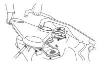
7 Loosen the spring that tensions the V-belt and pry off the belt.
