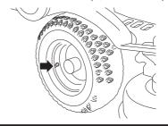
IMPORTANT! Different tyre pressures on the front tyres will result in the blades cutting the grass at different heights.
