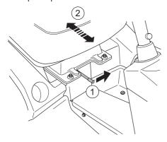
The seat springing can be adjusted by moving the rubber stops in their mountings on the underside of the seat. Place both stops in the front, middle or rear.
