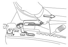
In order to ensure that the hydraulic cylinder is in the outer position, hold the lever in the forward position for a half to one second.
