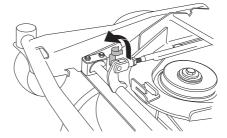
Remove the bolt so the track rod is released in one end.
