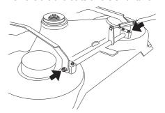
6 Remove the screws on the cutting cover. Lift the unit frame and remove the cutting unit cover.
