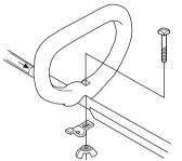
• Now adjust the trimmer to give a comfortable working position. Tighten the wing nut.
