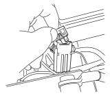
Do not use any other type of fuse when replacing.
