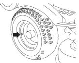
CAUTION! Different tyre pressures on the front tyres will result in the blades cutting the grass at different heights. Having the same air pressure in the tyres is important in order to achieve the best possible performance as well as to avoid damage to the machine
