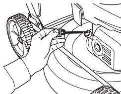
Place a suitable vessel to collect the oil in.
