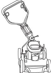
The handle can also be adjusted vertically by turning the wheels by the attachment fitting on the chassis
