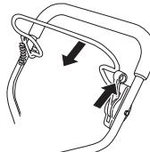
The engine brake should always be adjusted so that the engine stops within 3 seconds.
