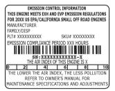
The Emissions Compliance Period referred to on the Emission Compliance label indicates the number of operating hours for which the engine has been shown to meet Federal and California emissions requirements.
