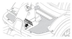
The pedal can also be used to temporarily adjust the cutting height, such as when passing a minor bump in the lawn.
