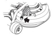
4 Fit the cutting deck's pipe together with the deck frame's pipe.
