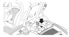
Check that the cooling intake is free from leaves, grass and dirt.
