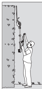
Vertical trimming at high level: Telescopic tube extended
