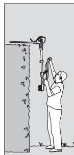
Horizontal trimming at high level: Motor unit tilted by 75°, telescopic pipe extended
