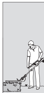
Trimming at low level: Motor unit tilted by -60°, telescopic pipe extended
