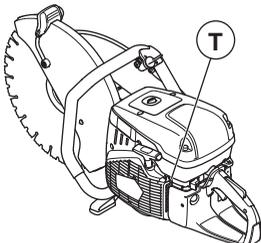
Rec. idle speed: 2700 rpm
