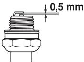
**NOTICE!** Always use the recommended spark plug type! Use of the wrong spark plug can damage the piston/cylinder.
