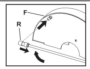
Install Water Pump (U): Unpack Water Pump (U) from its shipping carton. Install Water Pump (U) by plugging its Electrical Cord (NN) into the electric motor pigtail cord on the electric motor. Install the hose barb fitting onto the Water Pump (U), then push on the Water Pump Hose (S). Route Water Hose & Electrical Cord (NN) above the cross-brace of the Pan Weldment (B) to avoid contact with blade during operation. Place Electric Water Pump (U) in bottom of Pan Weldment (A).
