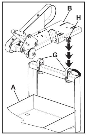
Pivot left and right Bearing Clamps (G) into their upper position. Tighten Knobs (K) until Bearing (H) of Head Platform (B) is secured into Pivot Block (J) of Pan Weldment (A).
