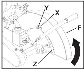
Install Tilt Arm (R) onto Blade Guard (F). Pivot Tilt Arm (R) upward until near Stud on Blade Guard (F). Pull collar on Tilt Arm (R) toward rear of machine, then connect with Stud on Blade Guard (F).
