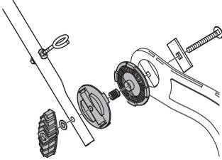
Use enclosed straps to secure cables to the handle. Do not overstretch cables when mounting.
