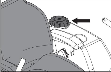
Read the safety instructions before refueling. The capacity for the tank is 5 gallons.
