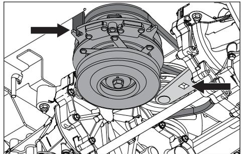
5. With the idler arm in the slack position, slip a screwdriver, clevis pin or similar into the 9.525 mm hole in the plate that sits between the two fan covers. This will keep the idler in the extended position and allow removal of the breaker bar.
