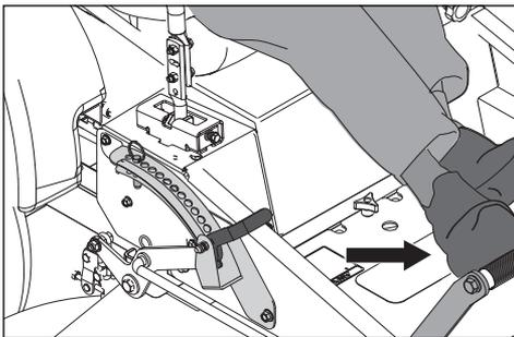
3. Activate the park brake, pulling the lever upwards.
