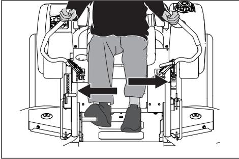
Make daily inspections to ensure that the safety system works by attempting to start the engine when one of the conditions is not met. Change the conditions and try again.
