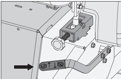
The park brake is found on the left of the machine. Pull the lever backward to operate the brake and push forward to release it.
