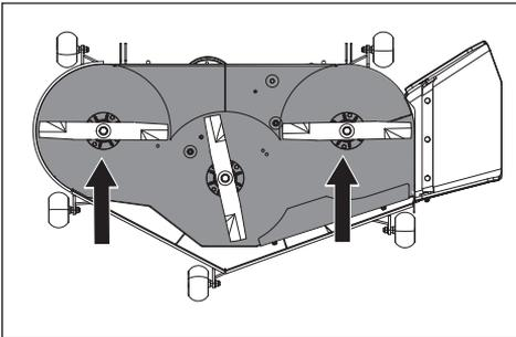
2. Measure from the floor surface up to the bottom of the blade tip on the discharge side of the mower deck. Record this measurement. Move to the opposite side; check that measurement is the same. If adjustment is required, loosen the locknut and adjust bolt up until both side-to-side measurements are equal. Retain measurement.
