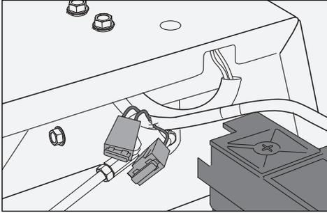
Fuses are located on the left hand side of the machine and are accessed by tilting the seat forward. Fuses are flat pin fuses type as used in automobiles. The 20 A is the primary fuse. The 7.5 A is for the mower deck coupling.
