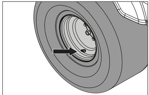
**IMPORTANT INFORMATION** DO NOT add a tire liner or foam fill material to the tires. Excessive loads created by foam filled tires will cause premature failures. Only use O.E.M. specified tires.
