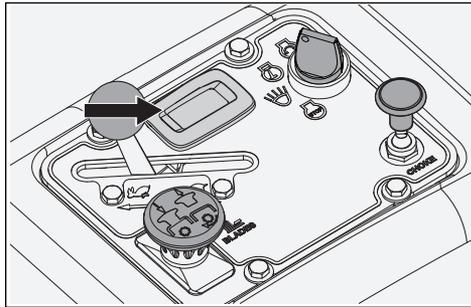
The service meter displays the total number of hours the engine has run and indicates when the engine and mower need servicing.
