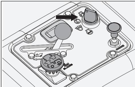
The ignition switch is placed on the control panel and is used to start and stop the engine. On models equipped with headlights, turn the key clockwise to ACCESSORY for headlight use.
