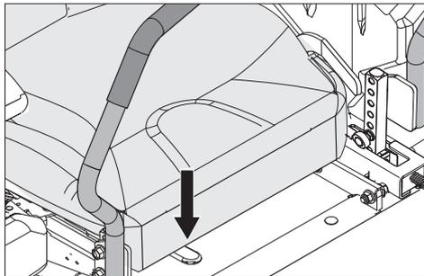
The seat can be adjusted lengthways. The lever under the front edge of the seat is moved to the left (as seen by the driver in the seat), to adjust the seat backward or forward.
