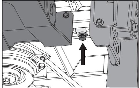
5. Allow the oil to fully drain from the engine.
