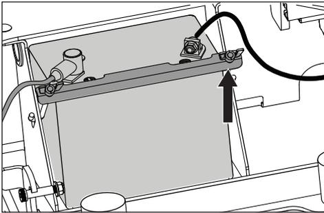
3. Using two 1/2" wrenches disconnect BLACK battery cable then RED battery cable.
