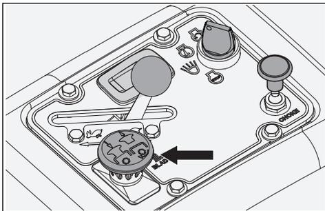
To engage the mower deck, pull the knob out; mower blades are disengaged when the knob is pressed down.
