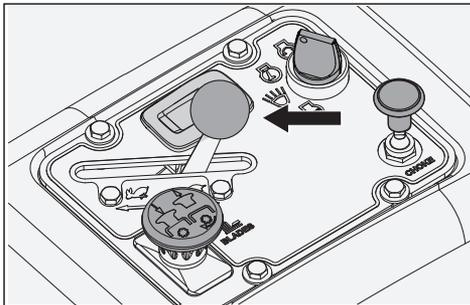
The throttle control regulates the engine speed and the rate of rotation of the blades, assuming the blade switch is pulled out.
