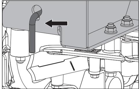
Transaxle bypass linkages must be engaged when pushing or pulling the mower. The release levers are located on each side of the rear of the unit below the rear engine plate. See **Manual Transport** in the *Operation* section.
