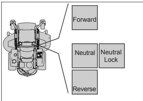
**WARNING!** The machine can turn very rapidly if one steering control is moved much further forward than the other.
