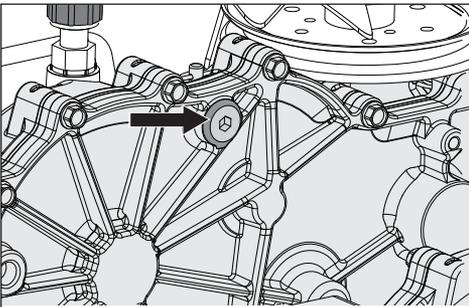
9. Remove the cap from the transaxles' expansion tank located on the vehicle frame.
