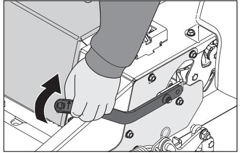
4. Push the blade switch down to disengage the mower blades.
