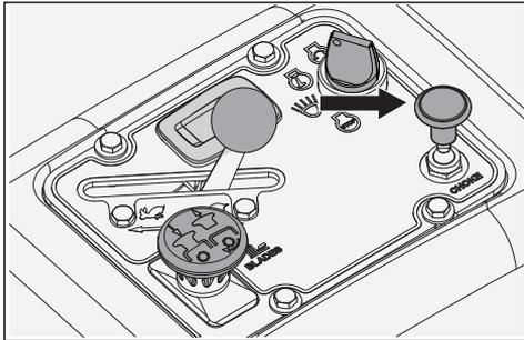
The choke control is used for cold starts to provide the engine with a richer fuel mixture. For cold starts, pull the control up.
