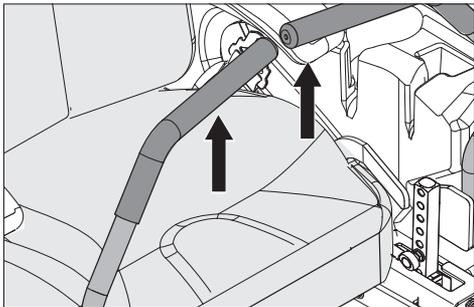
The machine's speed and direction are continuously variable using the two steering controls. The steering controls can be moved forward or backward about a neutral position. There is a neutral position, which is locked if the steering controls are moved out.
