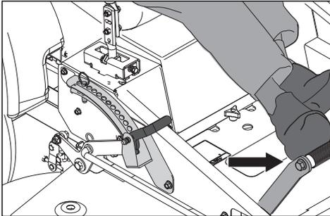
The desired cutting height is set with the height pin. The cutting height pedal releases the deck lift to place the deck at the selected height.
