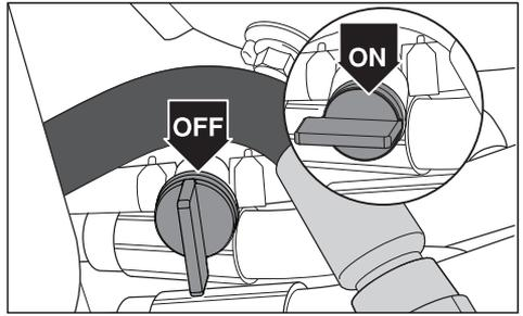
The fuel shut off valve is located at the left rear of the seat. The valve is off when the handle tab is turned perpendicular to the fuel line.
