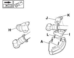
Remove the mounting plate (H). Fit the adapter (I) and bracket (J) with the two screws (K) as shown. Fit the blade guard (A) to the adapter using the 4 screws (L) as shown.
