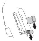
3 Push the equipment frame down and place the catch against the frame.
