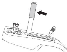
2 Move the throttle to the idle position. Turn the ignition key to the "STOP".
