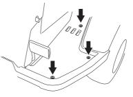
2 Loosen the locking nuts (1).
