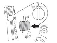
9 Set the required engine speed with the throttle control.
