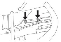
4 Screw out (extend) the stay to raise the rear edge of the cover.
