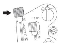
8 Let the engine run at moderate speed or half throttle for 3-5 minutes before subjecting it to heavy load.
