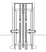
3 If necessary, the wires can be adjusted by tightening the adjuster nuts on each side of the steering collar.
