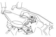
8 Loosen the spring that tensions the V-belt and pry off the belt.
