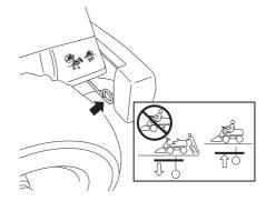
• Pull out the control to disengage the drive system. Push in the control to engage to the drive system.
