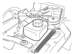
**Rider 316T** Fill if necessary with engine oil SAE 10W/40 (class SF–CC).
