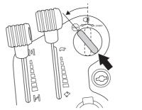
3 When the Rider is at a standstill, press down the parking brake and push in the locking button.
