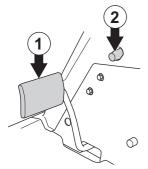
2 Carefully press down one of the pedals until the required speed is obtained. Pedal (1) is used to drive forwards, and pedal (2) to drive backwards.
