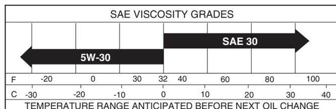
**NOTE:** Multi-viscosity oils (5W30, 10W30 etc.) improve starting in cold weather, and you should check your engine oil level frequently to avoid possible engine damage from running low on oil.
