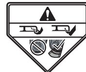
Warning! Keep away from the discharge deck, do not use without deflector or grass catcher
