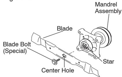
**IMPORTANT:** To ensure proper assembly, center hole in blade must align with star on mandrel assembly.
