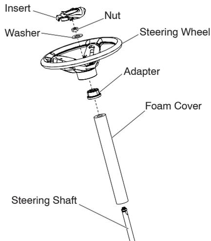
6. Remove steering wheel adapter from steering wheel and slide adapter onto steering shaft.
