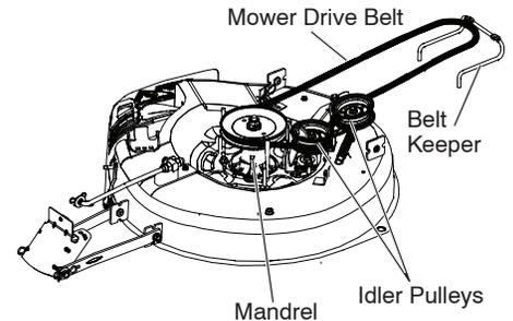
9. Check idler pulleys to see that they rotate freely.
