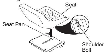
4. Pivot seat and pan forward and assemble adjustment knob and flat washer loosely. Do not tighten.
