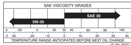
**NOTE:** Although multi-viscosity oils (5W30, 10W30 etc.) improve starting in cold weather, the oils will result in increased oil consumption when used above 32°F/0°C. Check your engine oil level more frequently to avoid possible engine damage from running low on oil.
