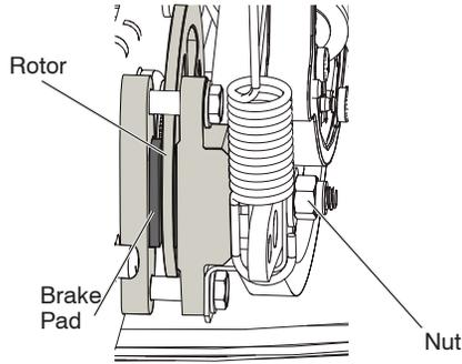
**NOTE:** Feeler gauge may be necessary to get correct measurement.
