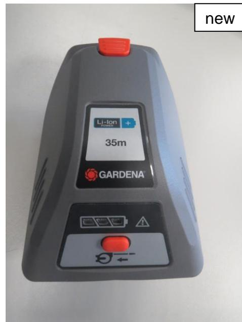
2. With index “J” new battery cells with higher capacity (2,2 Ah instead of 1,6 Ah) will be implemented for 2017. These batteries with higher capacity may only be charged with a new charger ( part. no. 8025-00.630.00 ), don't use the old one with part. no. 8840.00.630.00 !
