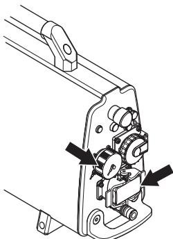
The other water connection should be connected to the power tool, the power tool has various regulating taps for regulating the flow of cooling water to the tool. See the operator's manual for the respective power tools.
