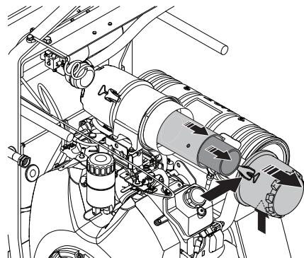
**CAUTION!** The 2 air filter housing clamps can not be closed unless the outer air filter is properly installed.
