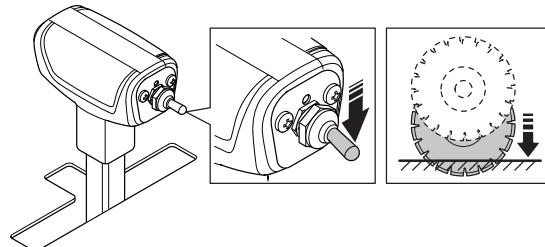
**CAUTION!** When lowering the blade into a partial cut, align the blade exactly with the cut to prevent damage to the blade.
