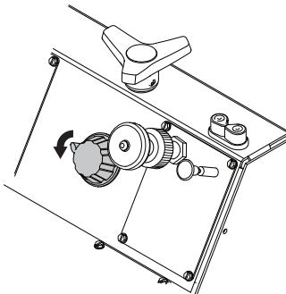
**CAUTION!** The touch should be smooth to prevent damaging the blade. Use Saw lowering speed control knob to slow down the lowering speed.
