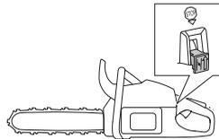
**NOTE!** The start/stop switch automatically returns to run position. To avoid involuntary start up, the spark plug cap must always be removed from the spark plug when the machine is unsupervised.
