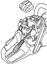
For temperatures below -5°C (23°F) and/or in snow conditions a special cover is available, which is mounted on the starter housing.
