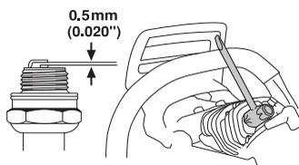
**Note!** Always use the recommended spark plug type! Use of the wrong spark plug can damage the piston/cylinder. Check that the spark plug is fitted with a suppressor.
