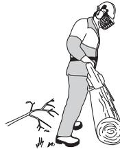
Keep the trunk between you and the chain saw as you move along the trunk.
