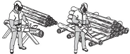
**The log is lying on the ground.** There is little risk of the chain jamming or the object splitting. However there is a risk that the chain will touch the ground when you finish the cut.
