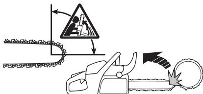
Cutting with the bottom edge of the bar, i.e. from the top of the object downwards, is known as cutting on the pull stroke. In this case the chainsaw pulls itself towards the tree and the front edge of the chainsaw body rests naturally on the trunk when cutting. Cutting on the pull stroke gives the operator better control over the chainsaw and the position of the kickback zone.
