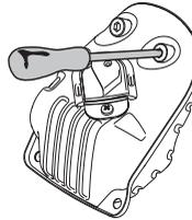
Some mufflers are equipped with a special spark arrester screen. If your machine has this type of muffler, you should clean the screen at least once a week. This is best done with a wire brush. A blocked screen will cause the engine to overheat and may lead to serious damage.
