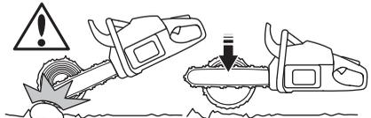
If it is possible (can you turn the log?) stop cutting about 2/3 of the way through the log.
