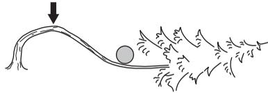
Decide which is the safest way to release the tension and whether you are able to do it safely. In complicated situations the only safe method is to put aside your chain saw and use a winch.
