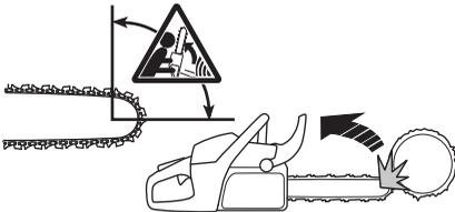
Kickback always occurs in the cutting plane of the bar. Normally the chainsaw and bar are thrown backwards and upwards towards the user. However, the chainsaw may move in a different direction depending on the way it was being used when the kickback zone of the bar touched the object.
