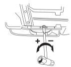
Recommended settings: Bar 13"-15": Minimum flow Bar 16"-18": Medium flow Bar 20"-28": Maximum flow
