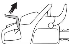
Never carry or hang the saw by the trigger! This could damage the mechanism and disable the chain brake.
