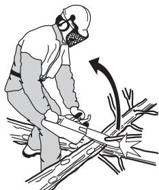
Have control over the workpiece. If the pieces you intend to cut are small and light, they can jam in the saw chain and be thrown towards you. Even if this does not need to be a danger, you may be surprised and lose control of the saw. Never saw stacked logs or branches without first separating them. Only saw one
