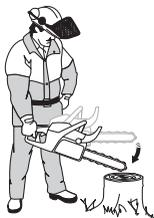
When the bar hits the stump the brake should be activated.
