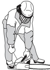
**CAUTION!** Do not pull the starter cord all the way out and do not let go of the starter handle when the cord is fully extended. This can damage the machine.
