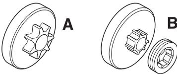
Regularly check the degree of wear on the drive sprocket. Replace if wear is excessive. Replace the drive sprocket whenever you replace the chain.
