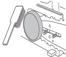
Regularly check that the brake band is at least 0,6 mm thick at its thinnest point.
