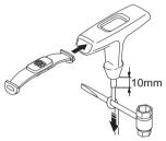
Assemble the starter and tighten the screws.
