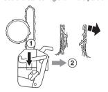
Next make the bottom cut so that it finishes exactly at the end of the top cut.
