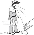
7 Take great care when cutting a tree that is in tension. A tree that is in tension may spring back to its normal position before or after being cut. If you position yourself incorrectly or make the cut in the wrong place the tree may hit you or the machine and cause you to lose control. Both situations can cause serious personal injury.
