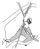
Gaining a good footing at the working position can be assisted by use of a temporary foot stirrup created from an endless sling.
