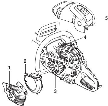
Clean the cooling system with a brush once a week, more often in demanding conditions. A dirty or blocked cooling system results in the machine overheating which causes damage to the piston and cylinder.
