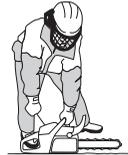
**Push down the red choke control** as soon as the engine fires which can be heard through a "puff" sound. Keep on pulling the cord powerfully until the engine starts.
