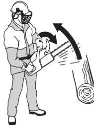
If the kickback is less violent or the kickback zone of the bar is closer to you the chain brake is designed to be activated manually by the movement of your left hand.
