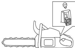
NOTE! The start/stop switch automatically returns to run position. In order to prevent unintentional starting, the spark plug cap must be removed from the spark plug when assembling, checking and/or performing maintenance.
