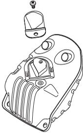
The muffler is designed to reduce the noise level and to direct the exhaust gases away from the operator. The exhaust gases are hot and can contain sparks, which may cause fire if directed against dry and combustible material.
