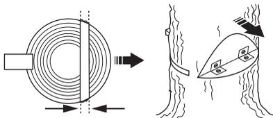
All control over the felling direction is lost if the felling hinge is too narrow or non-existent, or if the directional cuts and felling cut are badly placed.
