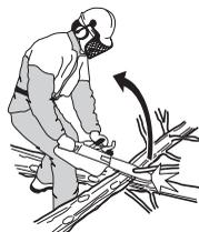
Have control over the workpiece. If the pieces you intend to cut are small and light, they can jam in the saw chain and be thrown towards you. Even if this does not need to be a danger, you may be surprised and lose control of the saw. Never saw stacked logs or branches without first separating them. Only saw one
