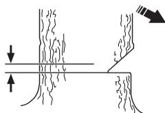
Finish the felling cut parallel with the directional cut line so that the distance between them is at least 1/10 of the trunk diameter. The uncut section of the trunk is called the felling hinge.
