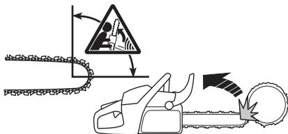
Cutting with the bottom edge of the bar, i.e. from the top of the object downwards, is known as cutting with a pulling chain. In this case the chain saw pulls itself towards the tree and the front edge of the chain saw body rests naturally on the trunk when cutting. Cutting with a pulling chain gives the operator better control over the chain saw and the position of the kickback zone.
