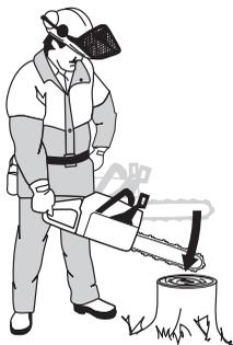
**When the bar hits the stump the brake should be activated.**
