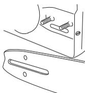
Tension the chain by turning the chain tensioning screw clockwise using the combination spanner. The chain should be tensioned until it does not sag from the underside of the bar.
