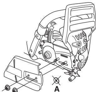
Fit the bar over the bar bolts. Place the bar in its rearmost position. Place the chain over the drive sprocket and locate it in the groove on the bar. Begin on the top edge of the bar.
