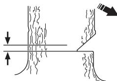
Finish the felling cut parallel with the directional cut line so that the distance between them is at least 1/10 of the trunk diameter. The uncut section of the trunk is called the felling hinge.
