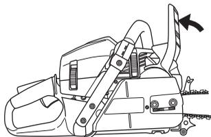
Remove the bar nuts and remove the clutch cover (chain brake). Take off the transportation guard (A).
