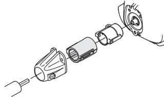
Regularly check the vibration damping units for cracks or deformation. Check that the vibration damping element is undamaged and securely attached.
