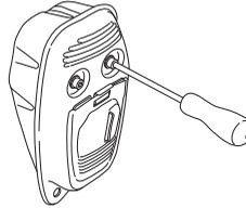
If the muffler on your machine is fitted with a spark arrestor mesh this must be cleaned regularly. A blocked mesh will cause the engine to overheat and may lead to serious damage.
