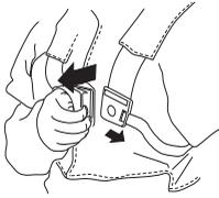
Check that the harness straps are correctly positioned. Once the harness and machine have been adjusted, check that the harness quick release works correctly.
