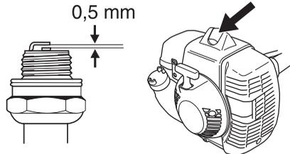
**CAUTION!** Always use the recommended spark plug type! Use of the wrong spark plug can damage the piston/cylinder.
