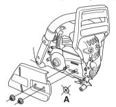
Fit the bar over the bar bolts. Place the bar in its rearmost position. Place the chain over the drive sprocket and locate it in the groove on the bar. Begin on the top edge of the bar.
