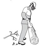
Keep the trunk between you and the chain saw as you move along the trunk.
