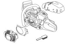
Clean the cooling system with a brush once a week, more often in demanding conditions. A dirty or blocked cooling system results in the machine overheating which causes damage to the piston and cylinder.
