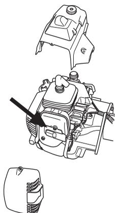
Some mufflers are equipped with a special spark arrestor screen. If your machine has this type of muffler, you should clean the screen at least once a week. This is best done with a wire brush.
