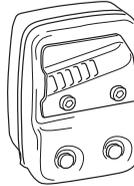
In countries that have a warm and dry climate there is a significant risk of fire. We therefore fit certain mufflers with a spark arrestor screen. Check whether the muffler on your machine is fitted with this kind of screen.
