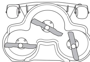
**CAUTION!** One or more unbalanced blades, caused by damage or poor balancing after sharpening, can cause vibrations in the machine.
