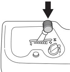
When the choke is engaged a richer fuel and air mixture is fed to the engine, which facilitates starting in the cold.
