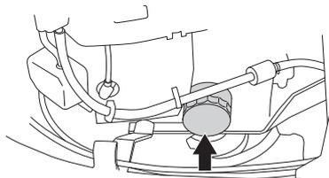
Lightly lubricate the rubber seal on the new oil filter using new oil. Fit the oil filter by turning clockwise. Turn by hand until the rubber seal is seated. Now tighten a further half turn.
