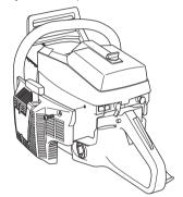
Clean the cooling system with a brush once a week, more often in demanding conditions. A dirty or blocked cooling system results in the machine overheating which causes damage to the piston and cylinder.
